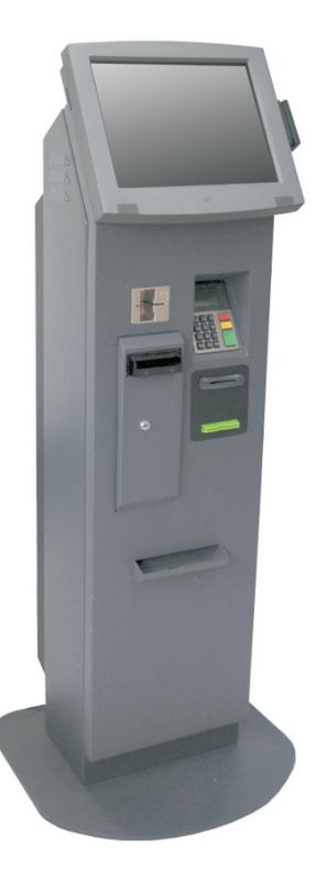
Smart3000-P Kiosk series is a multi-purpose device developed for users expecting high performance especially in payment system applications. The front-opening rack cover, large internal space and maintenance-friendly design provide significant advantages. The products is ideal for payment system solutions and projects such as ticket and coupon sales, purchasing phone minutes and paying bills thanks to its credit card payment and banknote acceptance mechanisms.
